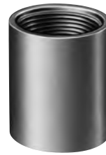
For adapting nonmetallic conduits to threaded fittings, metallic systems. Female threads on one end, socket end on other.
