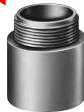
For adapting nonmetallic conduits to boxes, threaded fittings, metallic systems. Male threads on one end, socket end on other.
